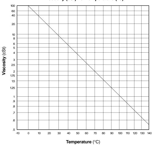
Fluorinert Liquid FC-70 Viscosity (cSt) vs. Temperature (°C)
